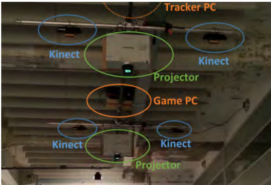
Figure 6.2: The hardware and construction for the Interactive Tag Playground at the art gallery.
